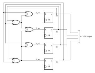
Figure 5: 4-bit Leap-forward LFSR
