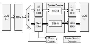
Figure 6: Proposed Module of Encoder/Decoder
