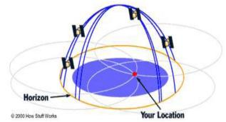
Figure 3: Principle of trilateration in 3-D space as used in GPS.
