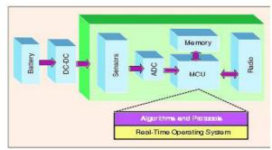
Figure 1. System architecture of a typical wireless sensor node
